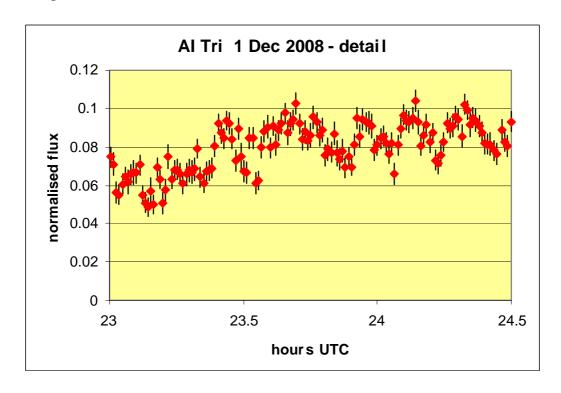
Flux is plotted on a linear scale, relative to an ensemble of comparison stars; a comparison at magnitude 15.6 is 0.093 on this scale. Error bars are  $1\sigma$ .
